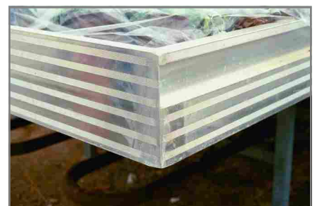
Welded and grinded corners
